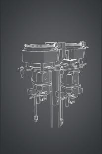
The Esprecious is fitted with the all new Bravilor Bonamat grinder. This patented grinder is extremely quiet and fast with low heat input. The steel grinder discs ensure the grind of the very first kilograms of coffee is just as constant as the next. While the renewed grinder outlet allows for an improved flow of coffee ground into the brew chamber.
